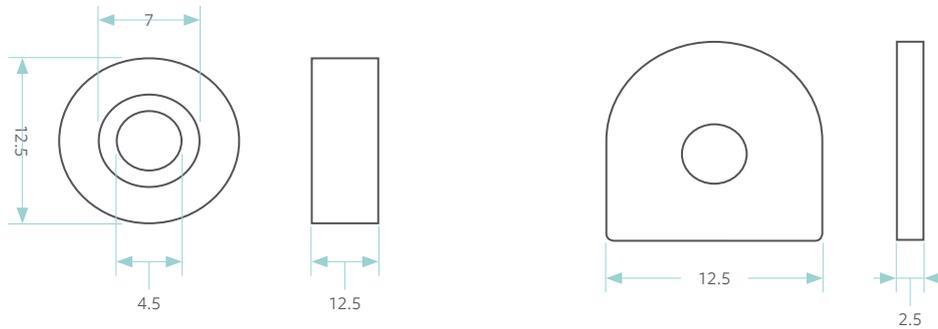
\*Magnets are attached to the shutter panel. Striking plates are attached to the frame.
